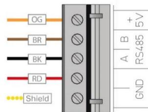
**Grounding** ⚠ **NOTE:** The metallic part of the housing of sensor must be connected to ground of machine by means of mounting or by shielded connection line!
