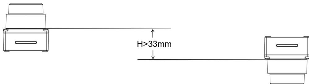
Figure 4 Multiple LiDARs bottoms placed opposite each other
