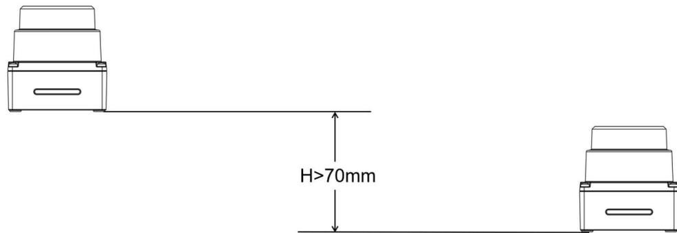
Figure 2 Multiple LiDARs forward placement
