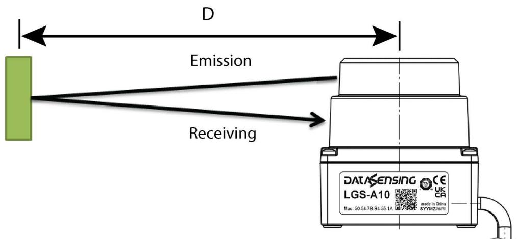
Figure 1 - LGS-A10 working principle
