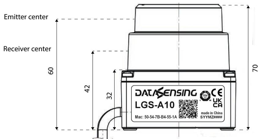
Figure 5 LGS-A10 light output position and receiving position
