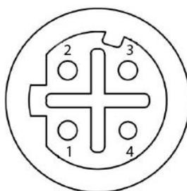
Figure 4 - Ethernet connector
