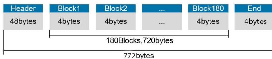
**Figure 1 - Format of point cloud information packet**
